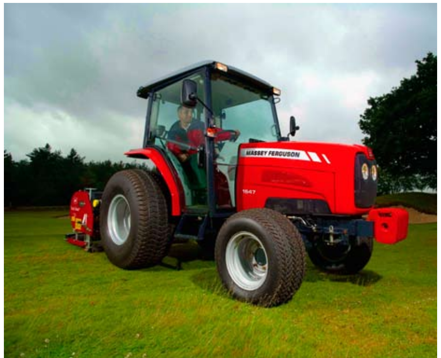
The Massey Ferguson Dyna QPS™ 12 forward/12 reverse transmission incorporates both a Power Shuttle and Power Shift which combines the positive drive of a three-range clutched gearbox with a clutchless change-on-the-move transmission.
