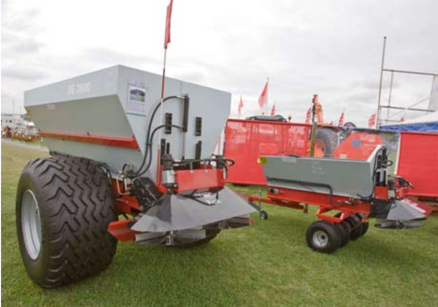
Trailed equipment, to include top dressers, are often offered with a choice of tyre size plus the option of two or four wheels across the rear of the unit. All this is wasted if the drawbar weight is transferred to the ground via skinny rear tractor tyres.
