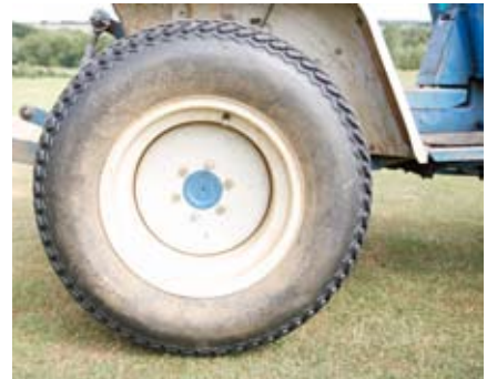
Some older tyre types are often inflated to needlessly high pressures. Try letting out some air, but mark the tyre and rim to check for tyre creep and look for any excess bulging. If the tractor has to carry a heavy load you may need to up the inflation pressure.
