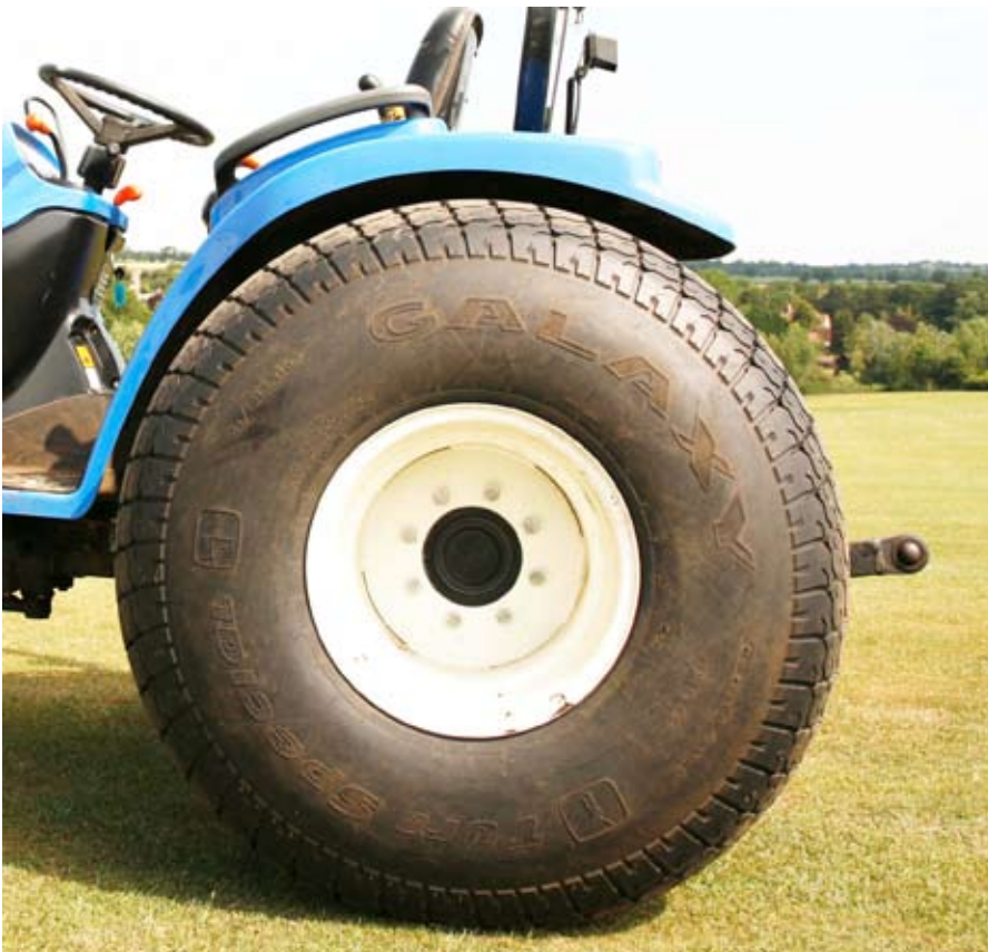
When looking to fit large flotation rubber to a tractor, seek advice. Fat tyres can foul mudguards and, if they have a different rolling diameter to standard, alter the tractor's gear ratios. Front and rear tyres need to be matched on 4WD models.
