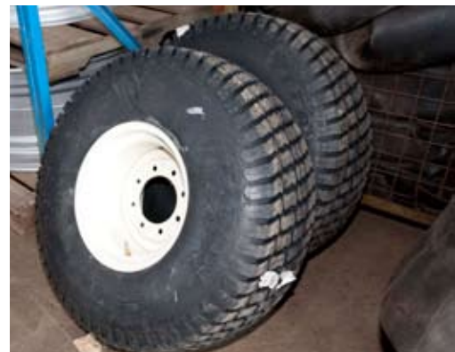
When considering alternatives to standard tractor tyre offerings, remember a wheel rim can have its central 'dish' position varied to allow a wider tread to be fitted with no risk of fouling the tractor's bodywork.
