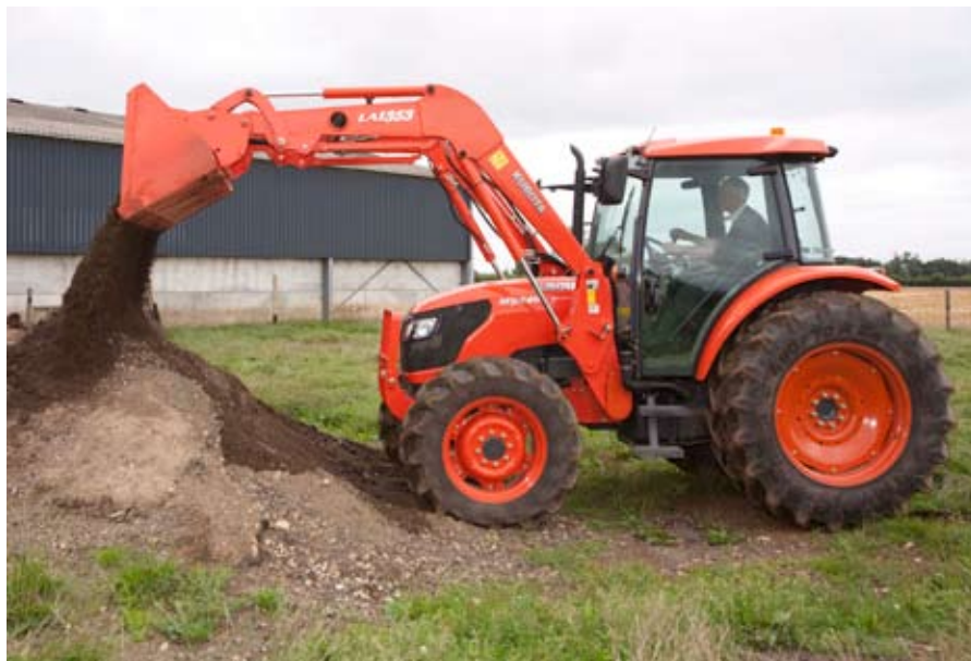
Standard agricultural pattern tyres can quickly destroy turf, but this type of tyre is often the best choice for general purpose duties...
