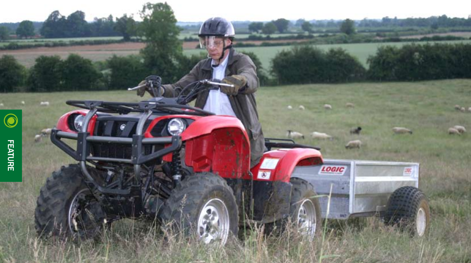
The agricultural sector has taken the ATV to heart, livestock farms in particular exploiting the ability of these units to get to hard to access parts of most farms. Note the use of gloves, hard hat and eye protection, a key basic requirement that should be adhered to.
