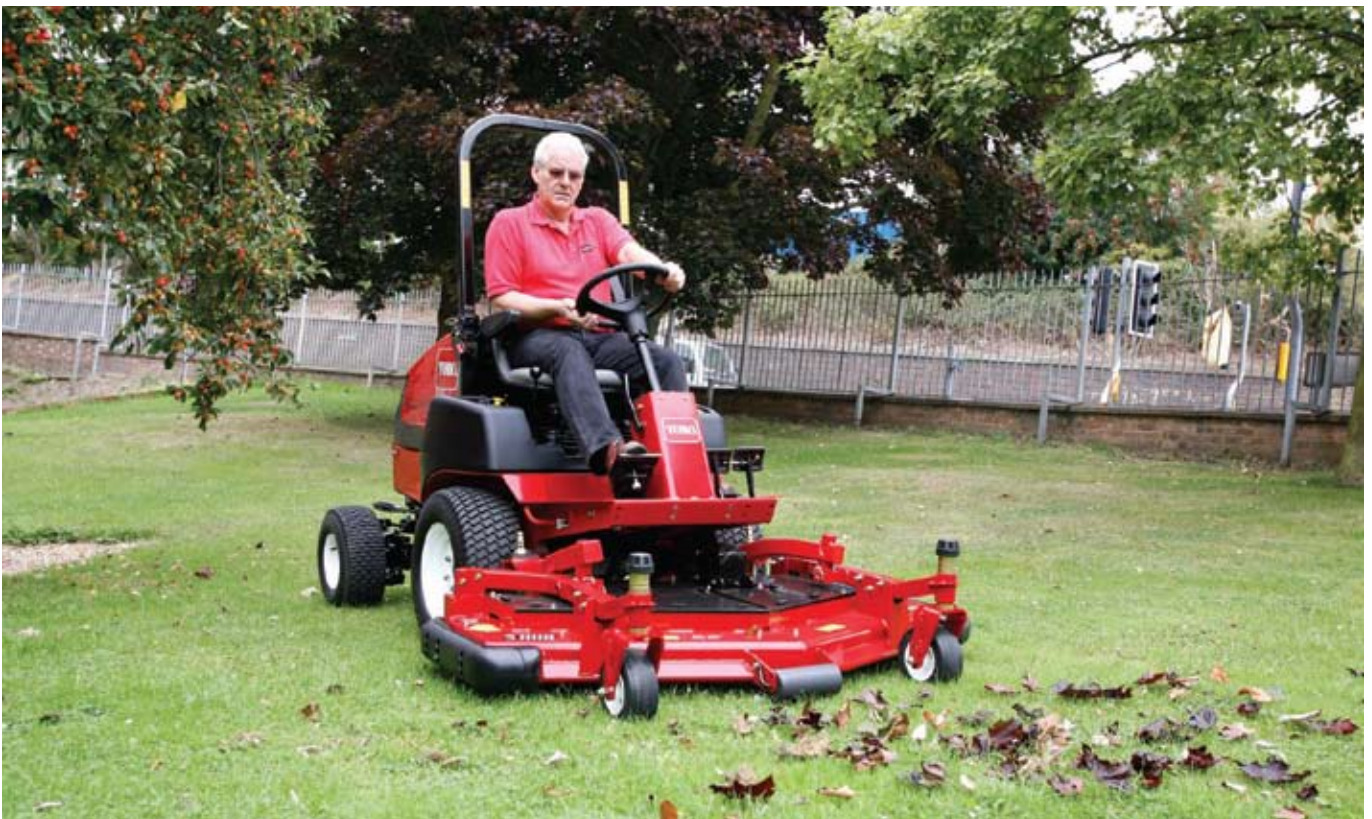
Toro traction management systems include its parallel hydraulic system. This delivers full-time, bi-directional 4WD, with parallel hydraulic flow between front and rear wheels. The system is designed to deliver more than just a traction boost in difficult conditions. During a turn, the wheels are also claimed to be less liable to scuff. As with all traction systems, it is how they can help protect the turf in difficult conditions that is as important to the ability to scale slippery inclines.
