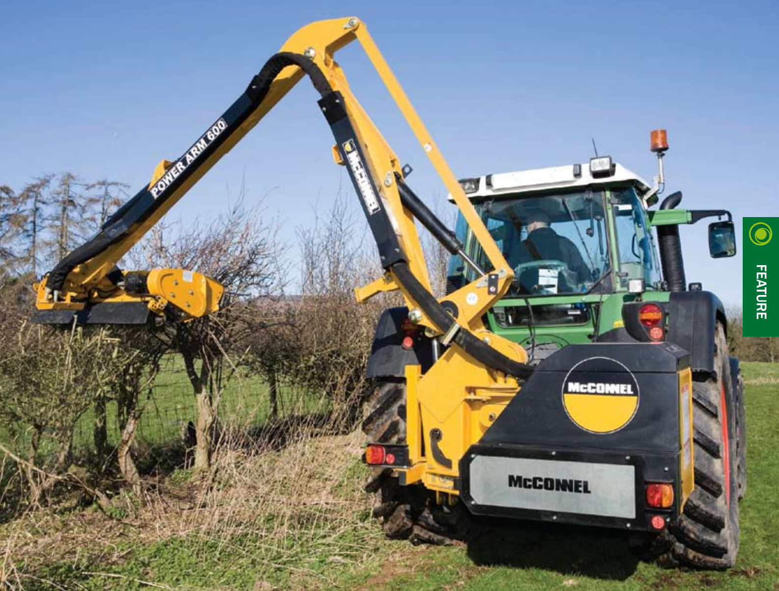
A tractor mounted flail hedge cutter will produce a clean cut on regularly maintained hedges, with the capacity to reduce a hedge to a manageable height even if it has been left uncut for several years. As a rule, the thicker the material a flail has to cut, the less attractive the finish will be. Pictured unit typically used by an agricultural contractor. Great for course boundary hedges.
