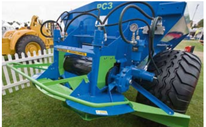
The design of top dressing equipment may be similar in outline but not in detail. The Pro-Cast PC3 from Sportsground Machinery drives its discs via hydraulically powered shafts. This keeps the hydraulic motors well out of the way of spread material. Spread width and patterns will vary according to the quality and quantity of top dressing applied, but a model like this is versatile; it will cope with large volumes of materials but will also spread light and thin if required.
