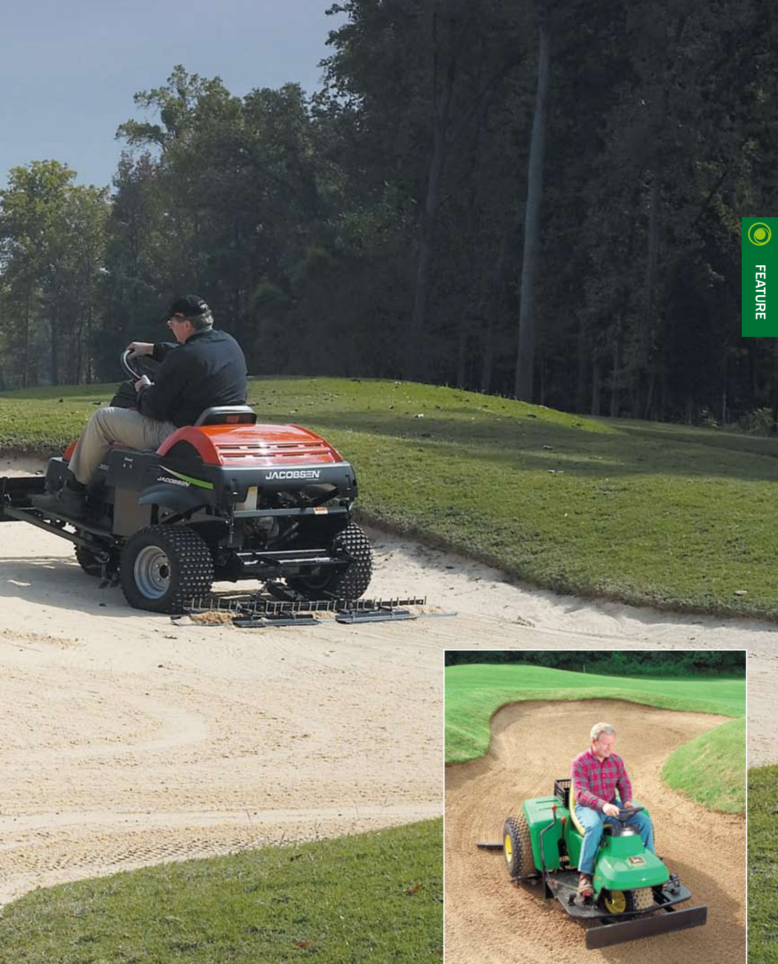
(Above) Simple to use, economical to buy and easy to look after, the John Deere 1200A bunker rake is well established in the UK. With its locking rear differential, the two-wheel drive 1200A has decent traction when needed and great manoeuvrability for tight bunker corners.
