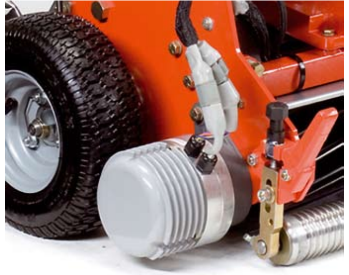
The electric direct-drive cylinder motor on the Jacobsen Eclipse 122 offers wider setting flexibility than a mechanical driven system
