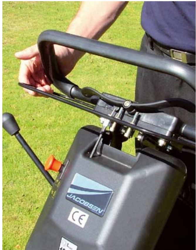
Familiar 'dead man' loop under D-handle has to be eased to the left and pulled up to engage the mower....
