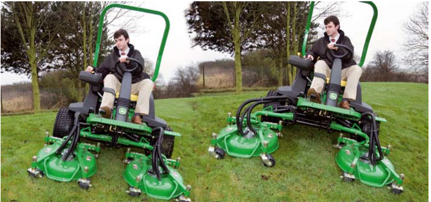
Powered by a 36hp turbocharged diesel, the all-new John Deere TerrainCut has three 27" decks. The 'Width on Demand' system enables the mowing width to be set at the standard 74" on level ground or reduced to a narrower 68". This will allow undulating ground to be mown with no fear of inter deck misses. All three wheels are powered to optimise traction
