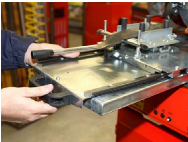
The carriage can be angled to allow the degree of blend grinding to be adjusted. This feature enables sharpening to be concentrated more at the blade tip and also reduces material removed from the blade shoulder, so retaining the blade's strength.
