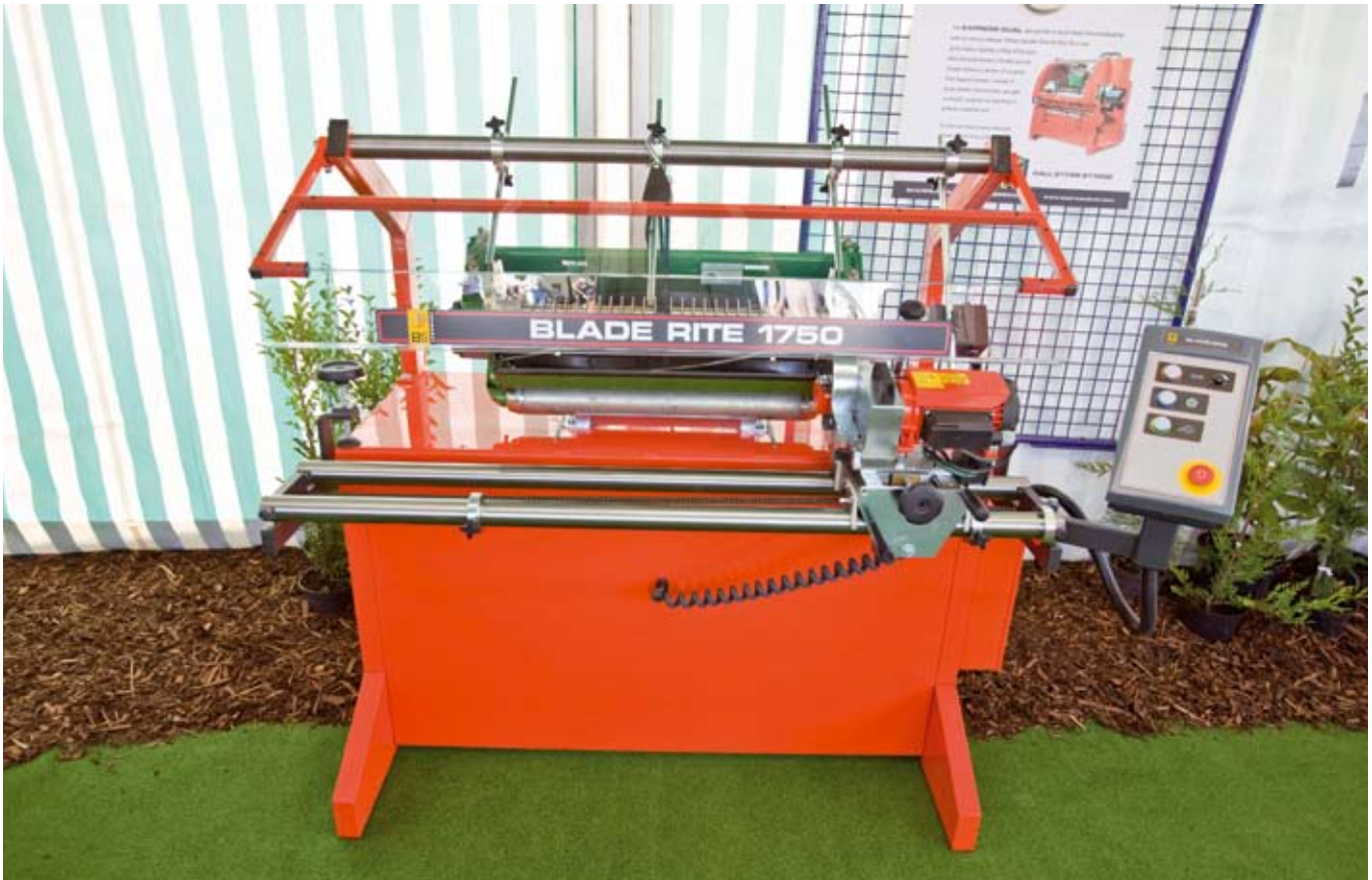
Modern grinding equipment includes models that are easier to set up and operate than some older designs, but that is not to say they can be used by just anybody. The Bernhard Blade Rite 1750 is among the easiest to set-up in the company's range, and can relief grind with the bottom knife in-situ.
