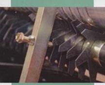
The setting bolt should just touch the groomer blade and then be taken back just a fraction to avoid contact
