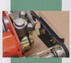
The belt of the rear roller brush drive should be checked to ensure correct tension
