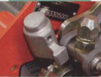
The course adjustment lever stops the grooming process. However, it continues to run and helps keep the grooved front roller free of debris
