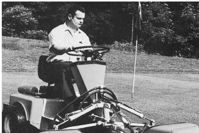
The Ransomes-Hahn Tournament Triplex was produced in the US, Ransomes importing it as a response to the Toro Greensmaster III. This first came to the UK in 1970 and was imported by Flymo International. In the USA, Jacobsen was the first to develop a ride-on greens mower in 1968. Powered by a 1.2hp petrol engine, the Ransomes-Hahn offered a 1.70m cut and could be supplied with verticutting, spiking and utility mowing reels. The first machine was sold in 1972, with 300 units having been sold by summer 1974
