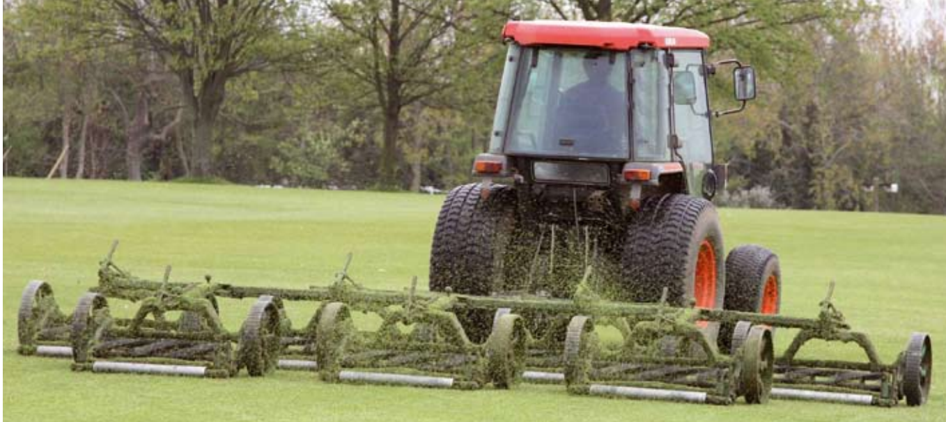
Gang mowers, such as the Lloyds Leda, remained the key fairway mowing tool until comparatively recently. Modern ride-on fairway mowers can now deliver a quality of cut that would have seemed far in excess of what was required back in 1977
