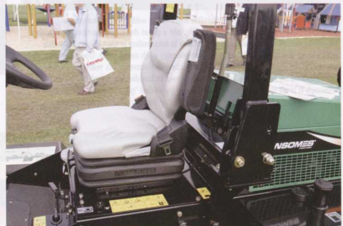
Seating remains something of a hot topic among operators; manufacturers sometimes offer a choice of seat but not necessarily with attractive enough pricing to tempt buyers to select the 'deluxe' option. Ransomes began to offer an air suspended seat as an option on its Highway models early this year. The value of this type of springing is not so much in added comfort but in the way the suspension automatically compensates for different operator weights. This is a real bonus on machines that may be operated by several different people. Fairway mowers will not really benefit from advanced suspension systems, but a seat that offers a good range of adjustment and support for the lower back is important. Larger tractors are offered with heated seats, an option that many would appreciate when mowing on a chilly morning
