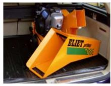
A 4hp Honda GC135 engine powers the 2008 production Primo. The unit can deal with material up to 1.5 in (3.8cm) in diameter, features a 60-litre collection bag and weighs just 35 kgs.
