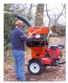
This powerful new model is equipped with 4 reversible heat treated steel chipper blades and a 76cm (30") diameter disc, driven by a 24hp Honda, which turns the disc at a remarkable 1500rpm via triple banded belt drive.
