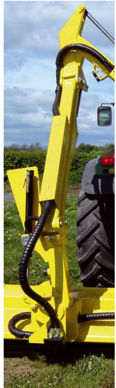
A Wiedenmann Super Pro TXL 1.8m side discharge rotary mower seen here linked to a Wiedenmann MCS XP 1500 collector
