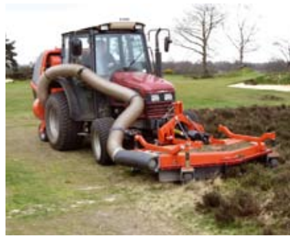
A Wiedenmann Super Pro TXL 1.8m side discharge rotary mower seen here linked to a Wiedenmann MCS XP 1500 collector
