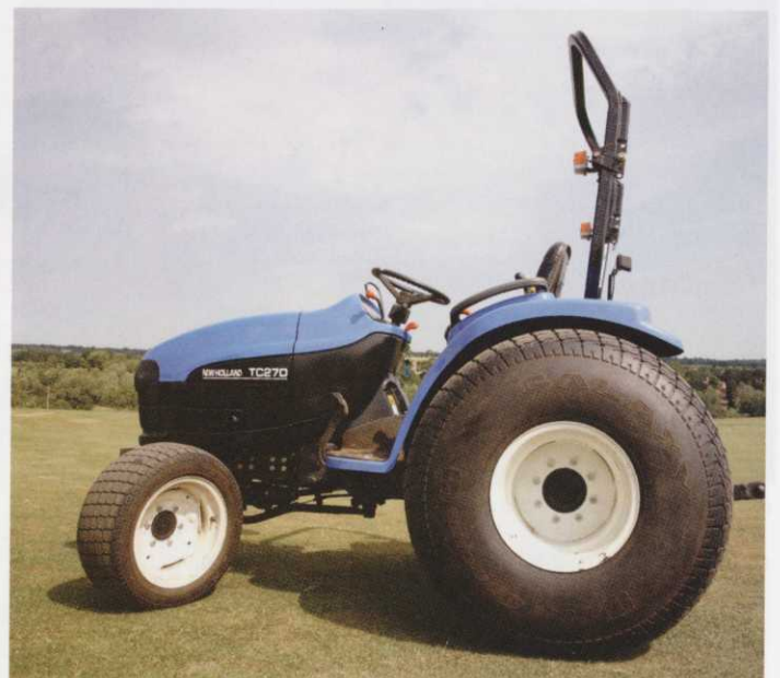
A tractor with 4WD can be extremely manoeuvrable. A flat tread at full lock is a point to look at as it will help reduce turf damage during a really tight turn. A simple test is to do a few 'doughnuts' with a demo tractor
