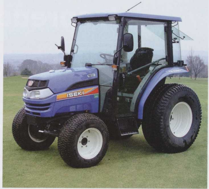
A modern tractor should be far less likely to leak oil, but accidents can happen. It is well worth using biodegradable oil in the hydraulics. This will not prevent hot spilt oil scorching the turf, but it will allow the damaged area to recover much faster
