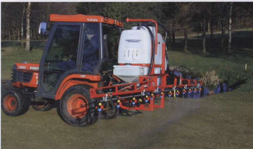
When spraying close to water ensure that LERAP guidelines have been followed and the correct nozzles have been fitted
