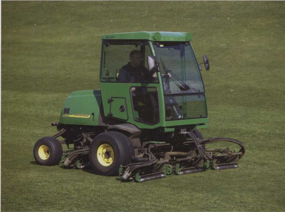
John Deere 3225C and 3235C models feature 22 inch cutting units, this now universally popular format being the size Deere has stuck to from day one. Cab option is increasingly popular, offering protection from the elements and stray balls
