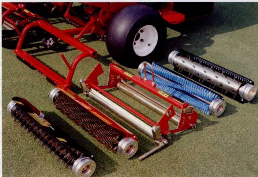
Cassette mounted equipment has opened the way for most greenscare operations to be done using a greens triple mower
