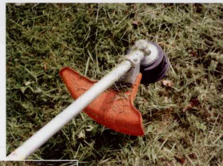
Grass cutting head, MB-KM, is the tool to select when using a brushcutter blade. STIHL offers a range of blade designs, including the twin blade pictured. In work, this left a clean cut, the cleared material appearing fair less mulched. "Normally we would use a star pattern blade, but the twin blade worked really well in long grass, leaving material that would be easier to rake up. Good guard"
