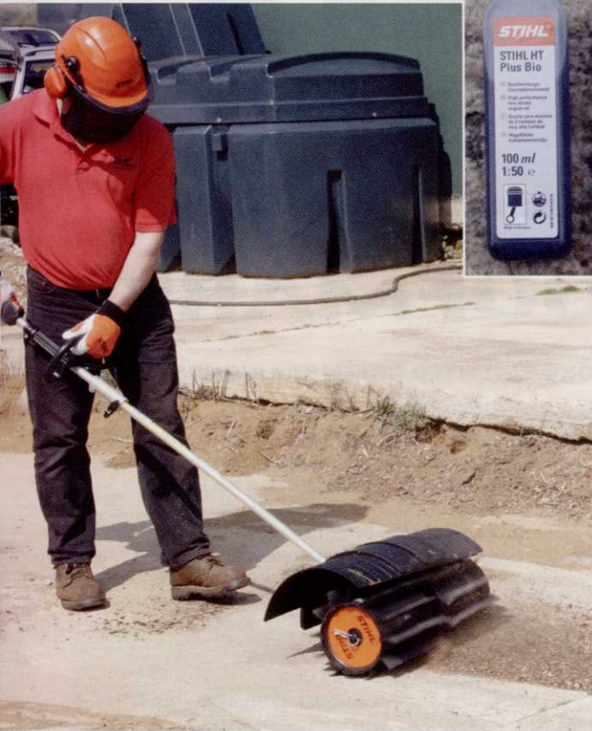
The rubber paddles of the KW-KM Power sweep have the advantage of not getting blocked when working with wet material. "The sweeping power of this unit, and the brush, is good and the tools are easy to operate"
