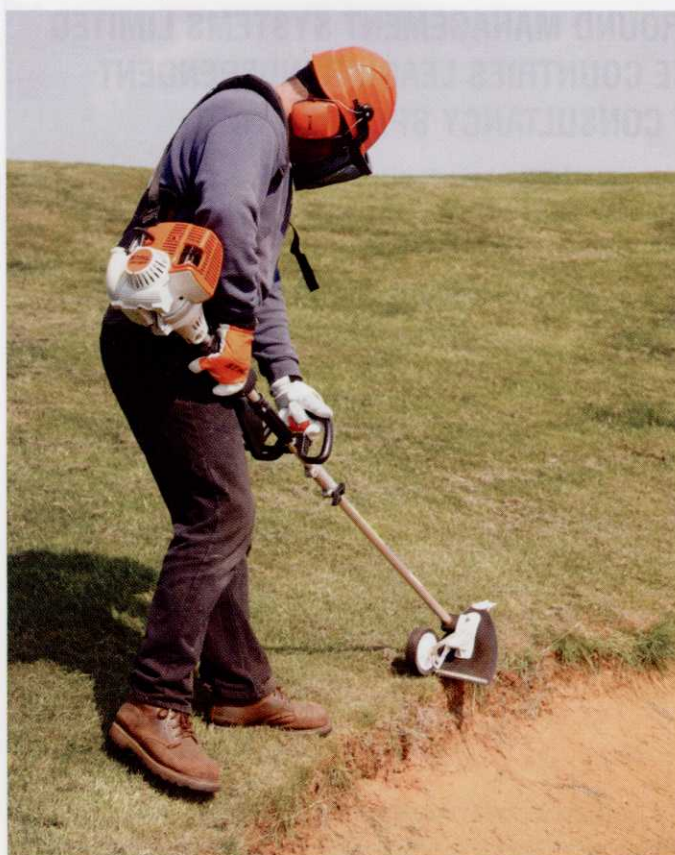
Designed predominantly as a Lawn edger, the FCB-KM unit was put to the task of trimming a bunker edge. It did a good job where the sand and grass were nearly level, but the Scrub cutter, or indeed manual edging shears, would be better for deep edges. "The jury is out on the value of this tool for bunker edging. I think it needs a bit of experience to get the best from too"
