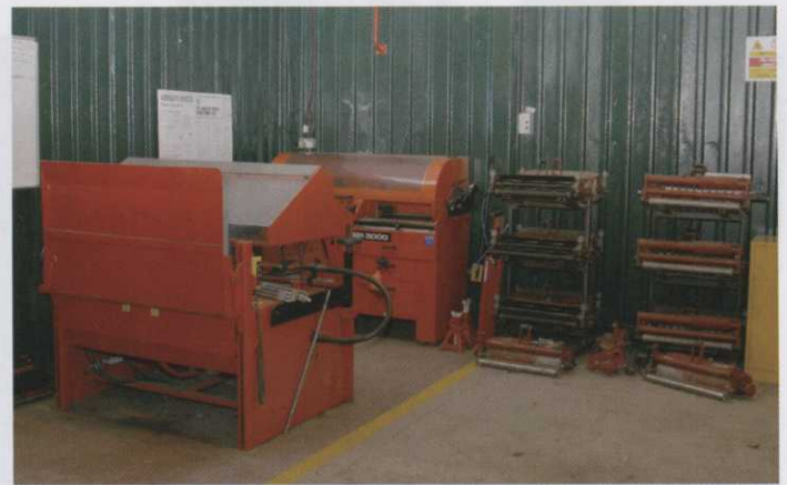
In-house cylinder grinding facilities are not unusual these days, but investing in sets of spare cutting units that are all set and ready to go remains less common. Money spent on good machinery support is never wasted
