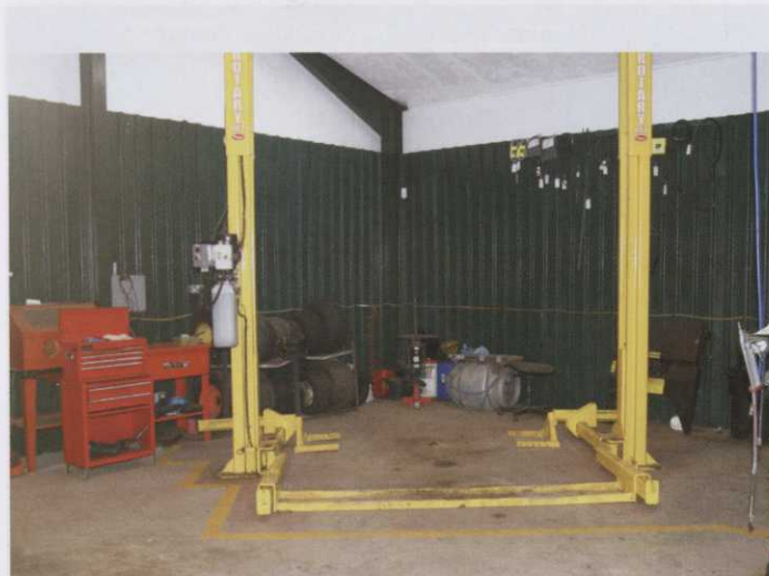
Modern vehicle lifts come in a wide range of capacities. Selecting the right design calls for a degree of forward thinking, but it always pays to have a degree of over capacity. Some lifts are more versatile than others
