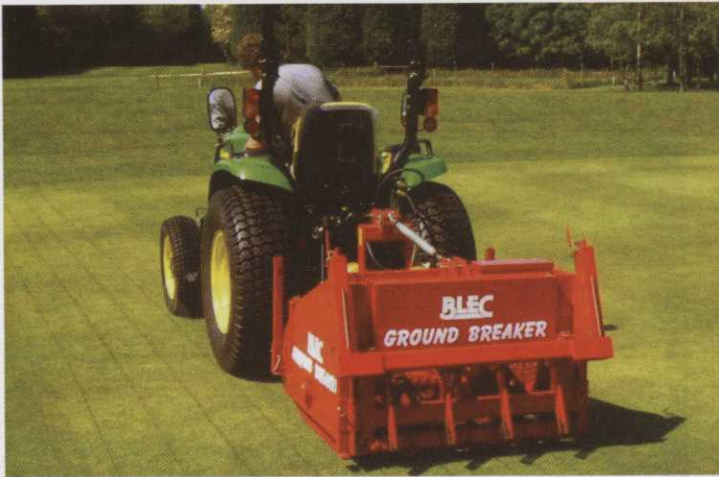
▲ Profound aeration creates countless millions of tiny cracks and fissures
