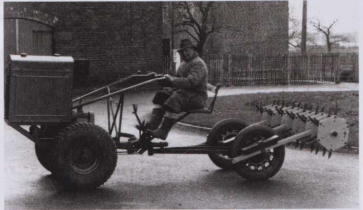
An early Sisis tractor mounted aerator. Scant protection from the elements both above and below
