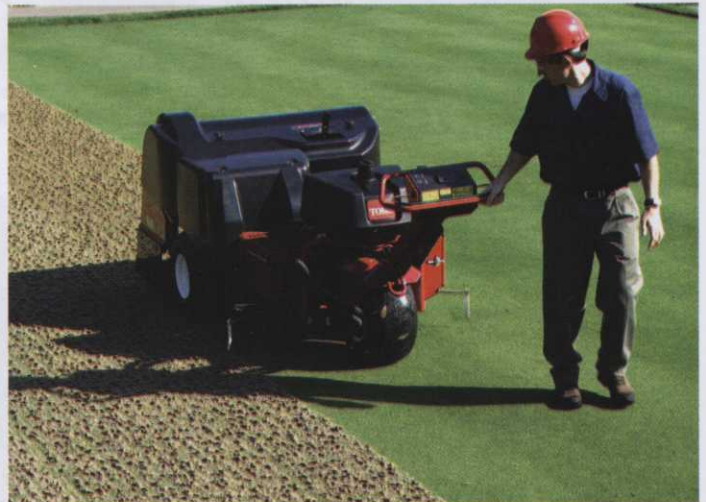
Toro's ProCore 648 can aerate 18 greens in just over seven hours according to the company
