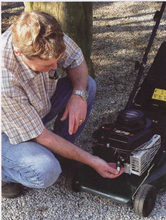
▲ Replace spark plugs as advised in the engine manufactures manual
