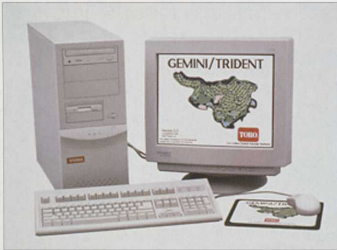
▲ PC-based irrigation control systems like this Toro Gemini-Trident unit offer major operational benefits to Course Managers and greenkeepers
