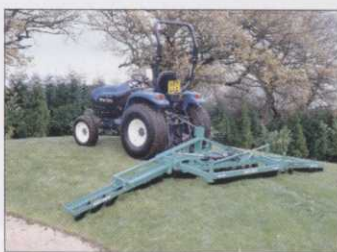
Three individual brush heads follow the contours of fairways and around your bunkers
