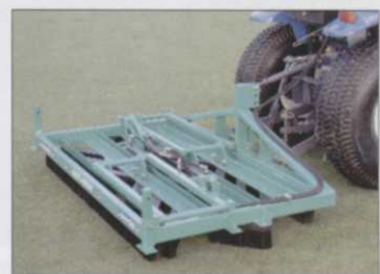
The Multi-Brush instantly transforms into a 6' wide zig-zag brush for greens
