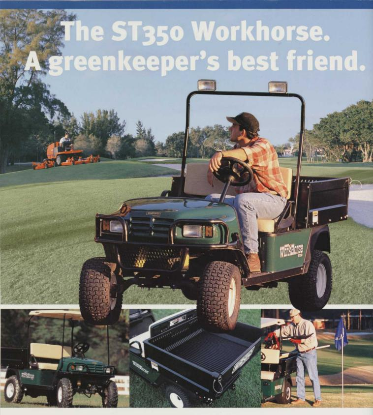
Whatever you want doing around the course the **ST350 Workhorse** is ready to help. Making light work of tough conditions. Speeding up **movement**, increasing **efficiency**. With its rugged 11hp engine, **heavy duty suspension** and tipping body the ST350 is a serious performer. Add the options of winch and worklights and you have all the capability you need to make a big impact on your workload. (And with the LPG version, a very **small impact on the environment**).
