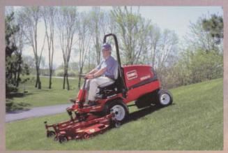
GROUNDSMASTER 223-D Highly-manoeuvrable and effortless to operate, the compact Groundsmaster 228-D with a 52in or 62in cutting deck, boasts a powerful new 28hp water cooled diesel Kubota engine, designed to give enough clout to tackle even the most challenging conditions.
