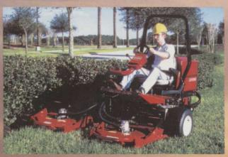
GROUNDSMASTER 3500-D SIDEWINDER Toro's unique Sidewinder rotary mower, with its innovative ability to shift the cutting units to the right or left, gives a quality finish right up to the bunker or water's edge. With a 35hp water cooled engine and three 27in floating rotary decks, its productivity is superb.
