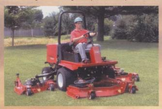
GROUNDSMASTER 4000-D Big, powerful and durable, Toro's 4000-D Groundsmaster won't let you down. Its 56hp engine combines with three decks to give a maximum cutting width of 11ft for great productivity over the toughest terrain.
