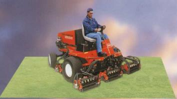
Resimaster 5500-D Fitted with a larger engine and bigger reel diameter for higher productivity, the 5500-D follows ground contours smoothly to give the finest of cuts. Options include 2 and 4 wheel drive, cab and grass boxes.
