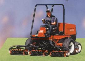
Reelmaster 6500-D A 38hp engine and larger reel diamet make this a highly productive and easy-to-operate fairway mower. Options include 2 and 4 wheel drive, cab and grass boxes.
