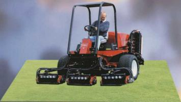
Reelmaster 6700-D Up to 11 feet of exceptional productivity is promised from the 6700-D's efficient 42hp engine, which comes with 4 wheel drive and is capable of cutting with 5, 6 or 7 units. Options include cab and grass boxes.
