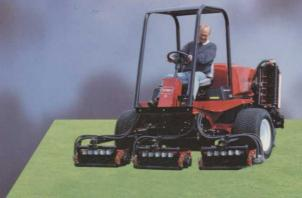
Reelmaster 6700-D Up to 11 feet of exceptional productivity is promised from the 6700-D's efficient 42hp engine, which comes with 4 wheel drive and is capable of cutting with 5, 6 or 7 units. Options include cab and grass boxes.
