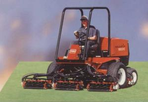
Reelmaster 6500-D A 38hp engine and larger reel diamete make this a highly productive and easy-to-operate fairway mower. Options include 2 and 4 wheel drive, cab and grass boxes.
