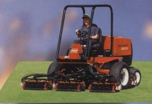
Resimaster 6500-D A 38hp engine and larger reel diameter make this a highly productive and easy-to-operate fairway mower. Options include 2 and 4 wheel drive, cab and grass boxes.
