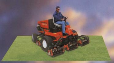
Realmaster 5500-D Fitted with a larger engine and bigger reel diameter for higher productivity, the 5500-D follows ground contours smoothly to give the finest of cuts. Options include 2 and 4 wheel drive, cab and grass boxes.
