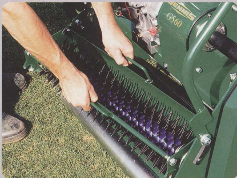
Below: Various attachments can be added using the cassette method
