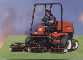
Reelmaster 6500-D A 38hp engine and larger reel diameter make this a highly productive and easy-to-operate fairway mower. Options include 2 and 4 wheel drive, cab and grass boxes.
