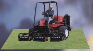
**Reelmaster 6700-D** Up to 11 feet of exceptional productivity is promised from the 6700-D's efficient 42hp engine, which comes with 4 wheel drive and is capable of cutting with 5, 6 or 7 units. Options include cab and grass boxes.
