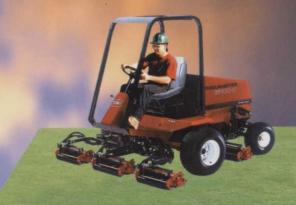
Reelmaster 5400-D Similar to its smaller stablemate, the 5400-D's larger 32hp turbocharged engine gives greater pulling power for more severe cutting conditions or steeper inclines.
