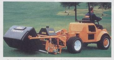
surface and leaving a clean finish. There is a high speed hydraulic motor on each unit while there are four interchangeable reels available: thatch removal reel; verticutting reel comprising close-pitched triangular blades for light scarification during the growing season; brush reel to remove light surface debris and lift grasses prior to mowing; combined reel with thatch removal blades interspersed with brushes to remove thatch.
