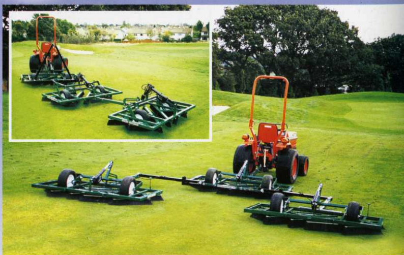
The 17' wide Triple Gang quickly grooms Fairways, stands up the grass before mowing, and disperses dew and worm casts.
