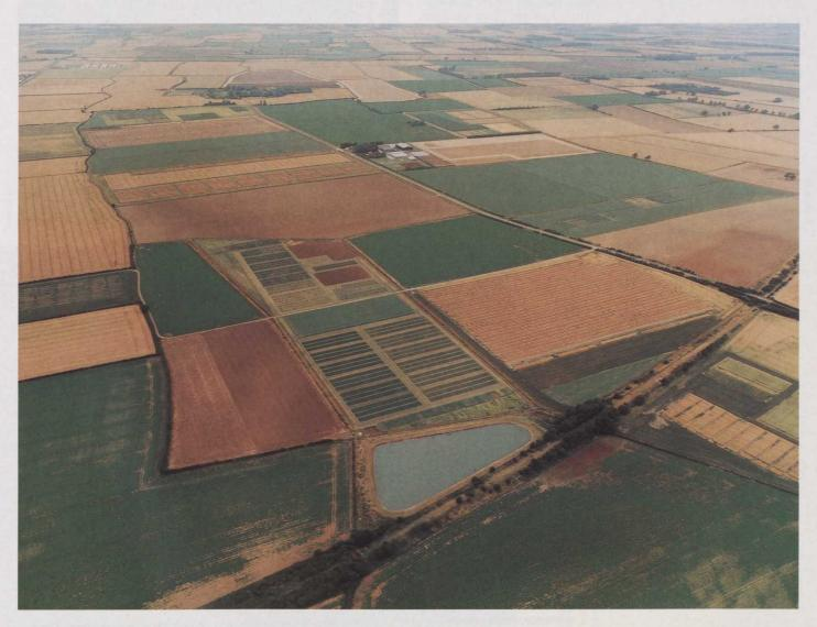
Above: An aerial view of Advanta's breeding, research and trial facilities at Boothby Graffoe near Lincoln. The recently constructed reservoir, which holds just under 23 million litres of water, enables the company to replicate average rainfall in times of drought.
