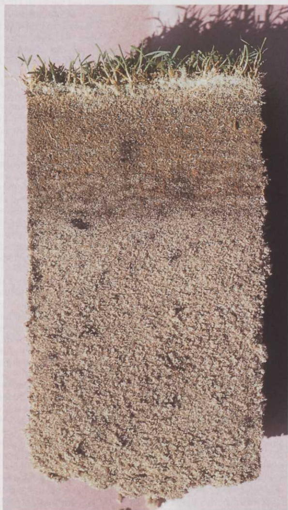
Above: A core sample taken from a predominately sand based green, which over the last five years, has received little thatch management
