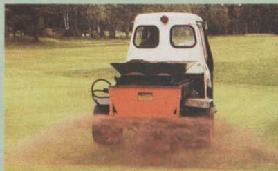
UB50 Precision Spreader. Truck mounted or trac- tor towed for greens and tees.
