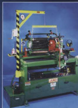
In Frame Juno 36" capacity cylinder and bottom blade grinding machine. Accurate 'relief' grinding of all cylinders, full in-situ capability, water cooled to suppress heat and dust. Cost effective, simple and fast!
