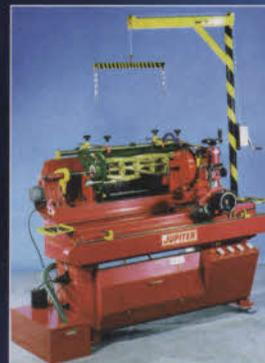
In Frame Jupiter 42" capacity cylinder and bottom blade grinding machine. Totally automated and water cooled as standard. A truly 'precision' grinder, built to last, used and preferred by professionals.
