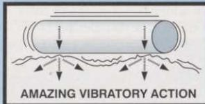
**TRUE-SURFACE** rollers weigh no more than your standard mowing units. Their unique vibratory action energises the surface particles and transforms the green back to its original shape without using a heavy roller!
