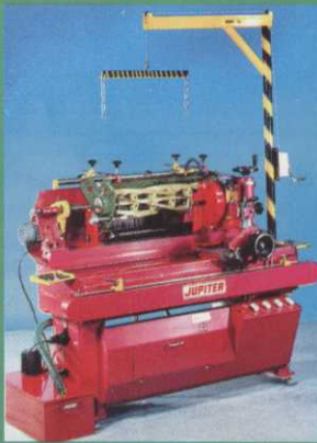
Jupiter. 42" capacity Mower Cylinder and Bottom Blade Grinding Machine. A truly 'precision' grinder, built to last half a century. Totally automatic and water cooled. Used and preferred by Professionals.
