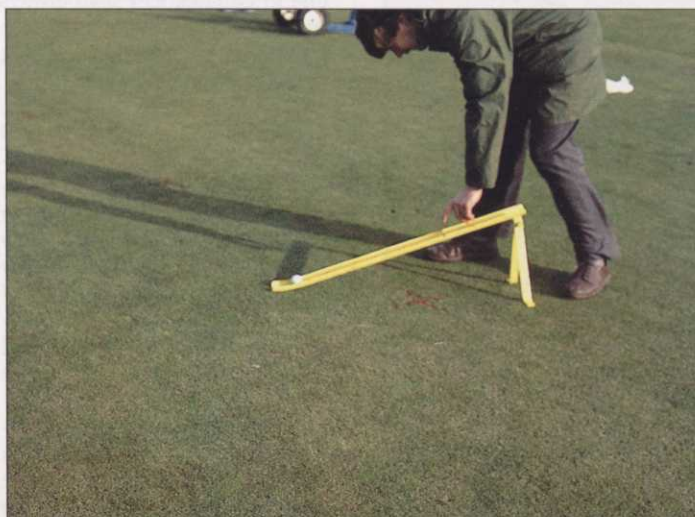
Measurement of green speed on a rootzone trial using an inclined ramp
