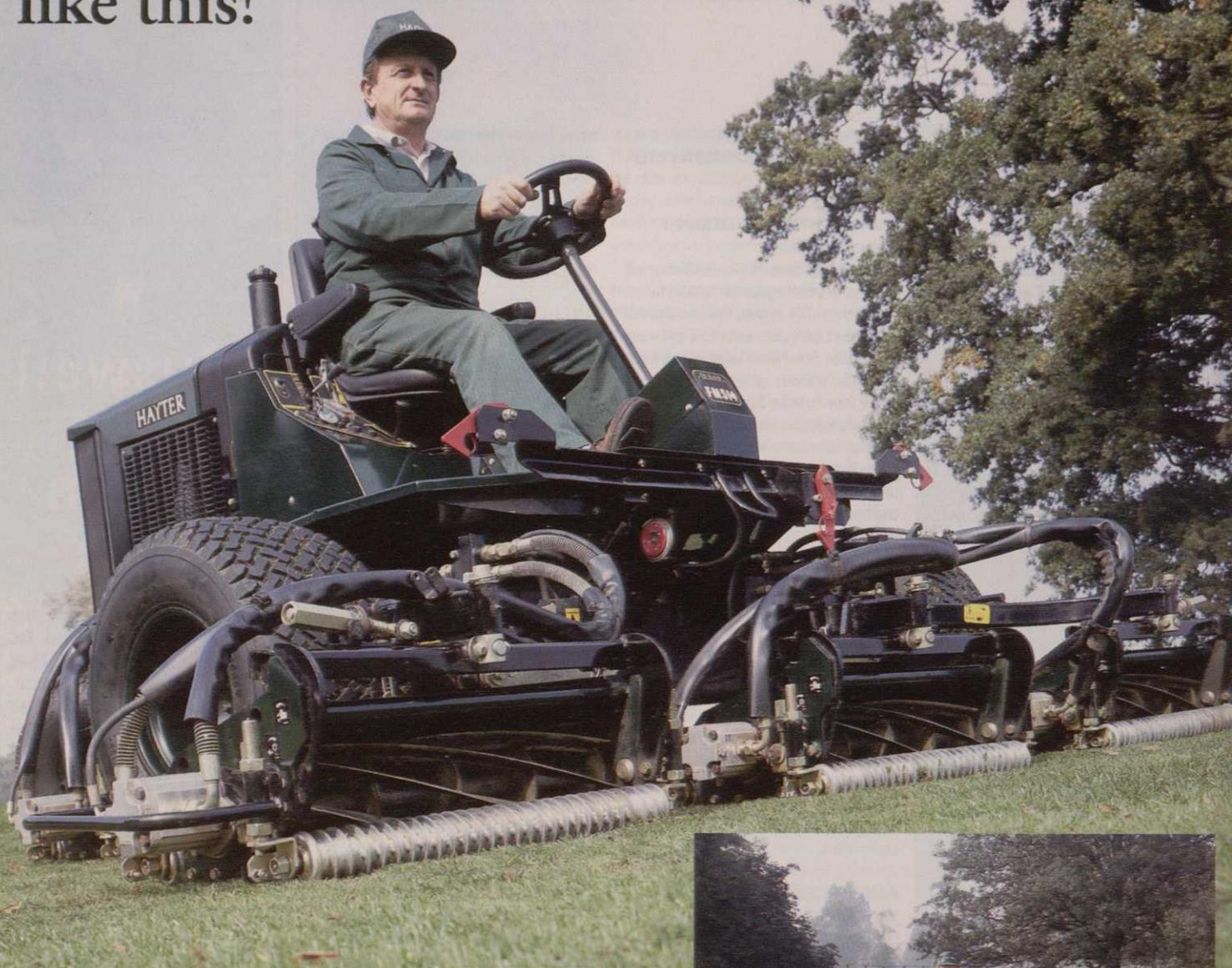
The Hayter FM514 is a purpose-built 5-gang mower that's equal to the challenge of any course. Since no two golf courses are the same, the FM is designed to adapt. Unique 26" floating heads follow the ground contours closely for a superb finish.
