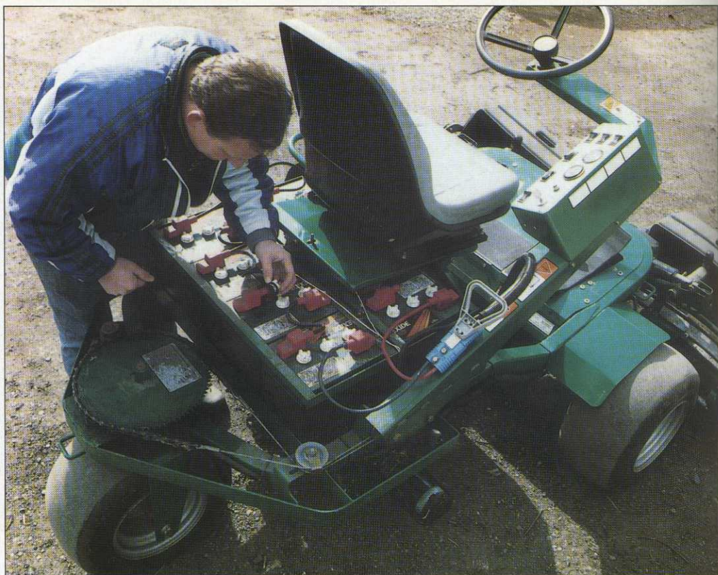
The E-Plex's batteries are checked daily by Paul Underhill, Head Greenkeeper at Brandhall Golf Club
