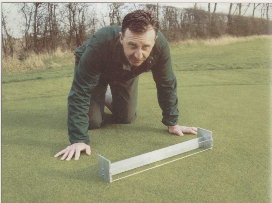
Philip Young, Head Greenkeeper at The Oaks, with an optical point quadrat frame
