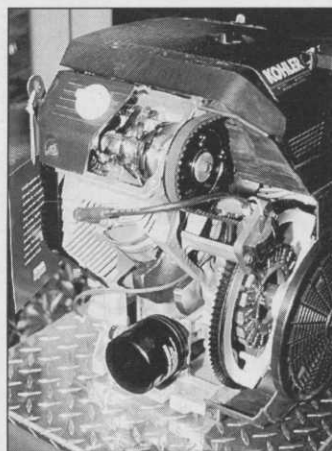
Cutaway of Kohler's 16hp V-Twin petrol engine with belt-driven overhead camshafts
