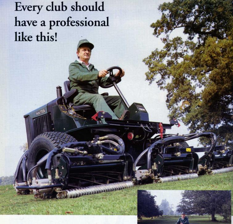
The Hayter FM514 is a purpose-built 5-gang mower that's equal to the challenge of any course. Since no two golf courses are the same, the FM is designed to adapt. Unique 26" floating heads follow the ground contours closely for a superb finish.
