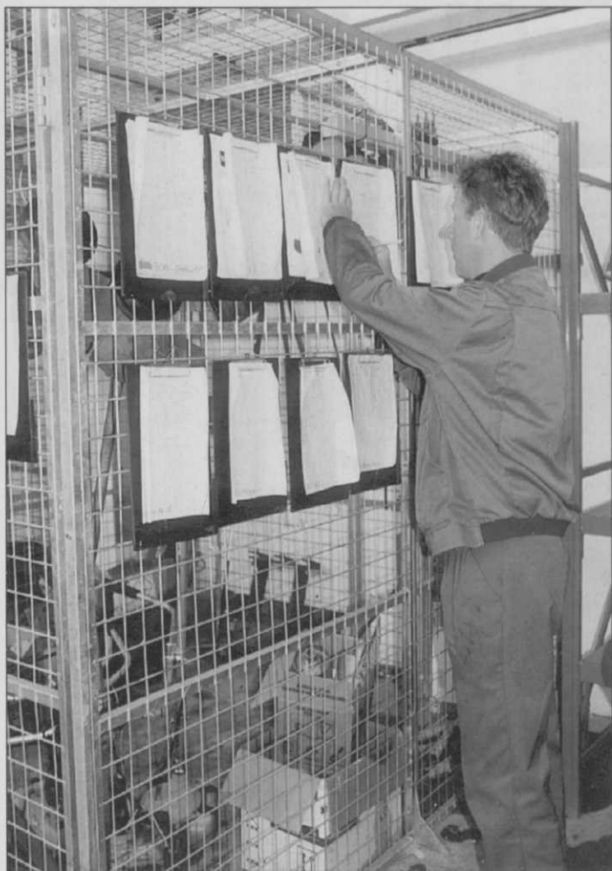
A check list is maintained for every machine. Note the security cage for storage of hand tools
