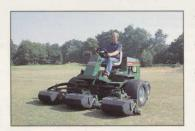
with a 38 horsepower engine. 4-wheel drive is standard except on 23hp model. Floating head cutting units closely hug
